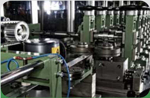
德国肖拉制管机 German Scholer Pipe Making Machine
